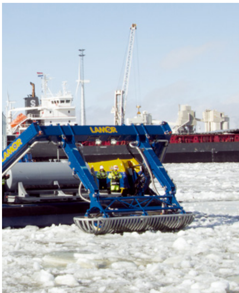
Sternmax 28, capacidad: 230 m 3 /h (1,012 gpm)
