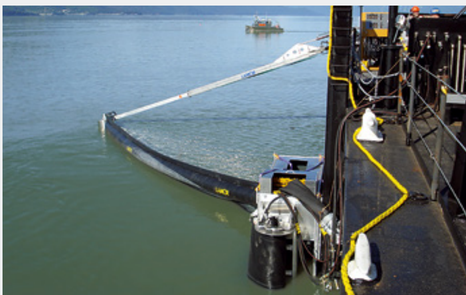
Recolector lateral / Casete lateral (LSC)
