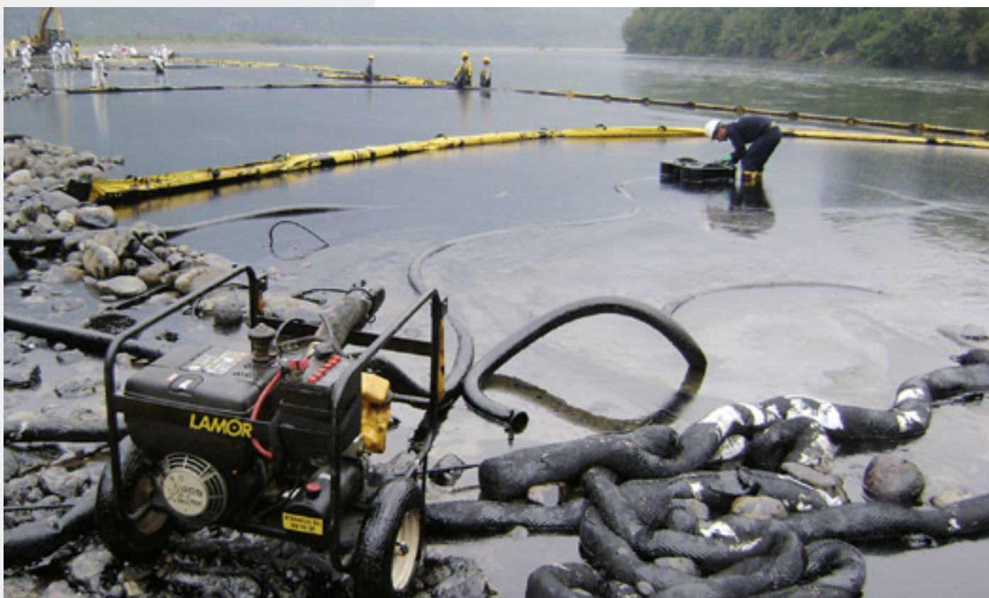
LPP 6 C75, potencia: 5.4 kW (7.2 hp)
