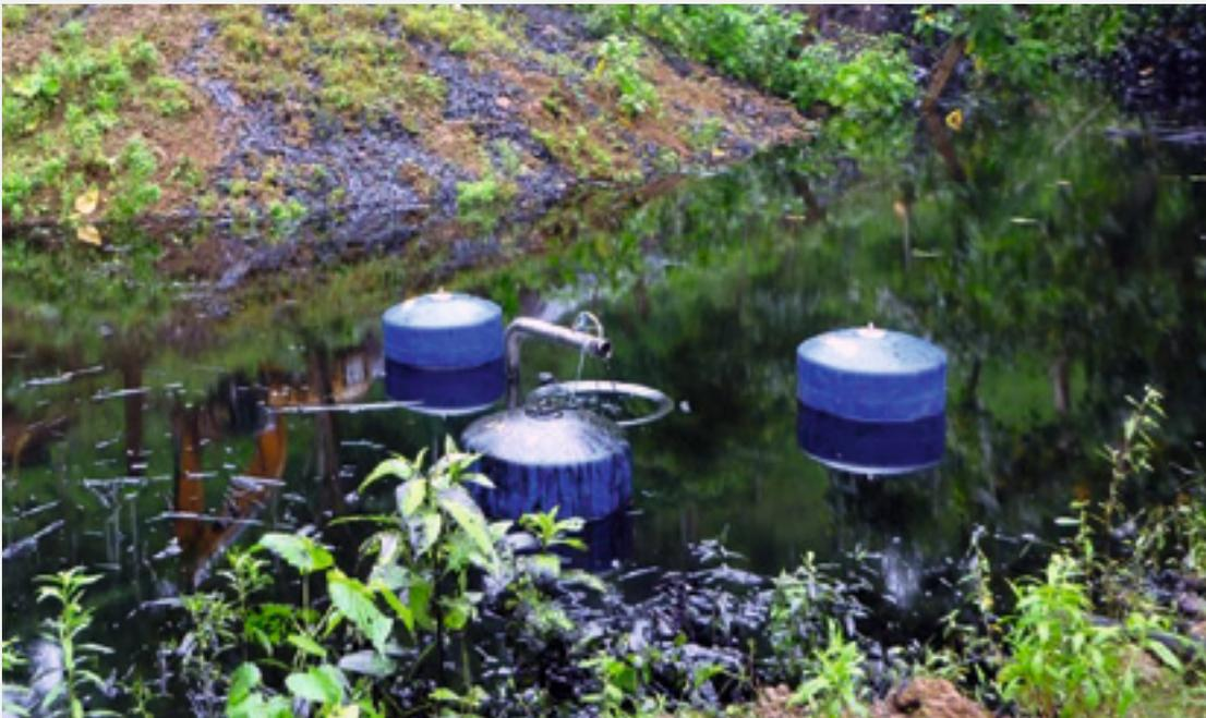
Weir skimmer 500, capacity: 70 m<sup>3</sup>/h (308 gpm)
