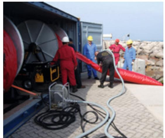
Inflatable Light Boom (PVC/PU & Neoprene), height: 650-1650 mm (26-65 in)
