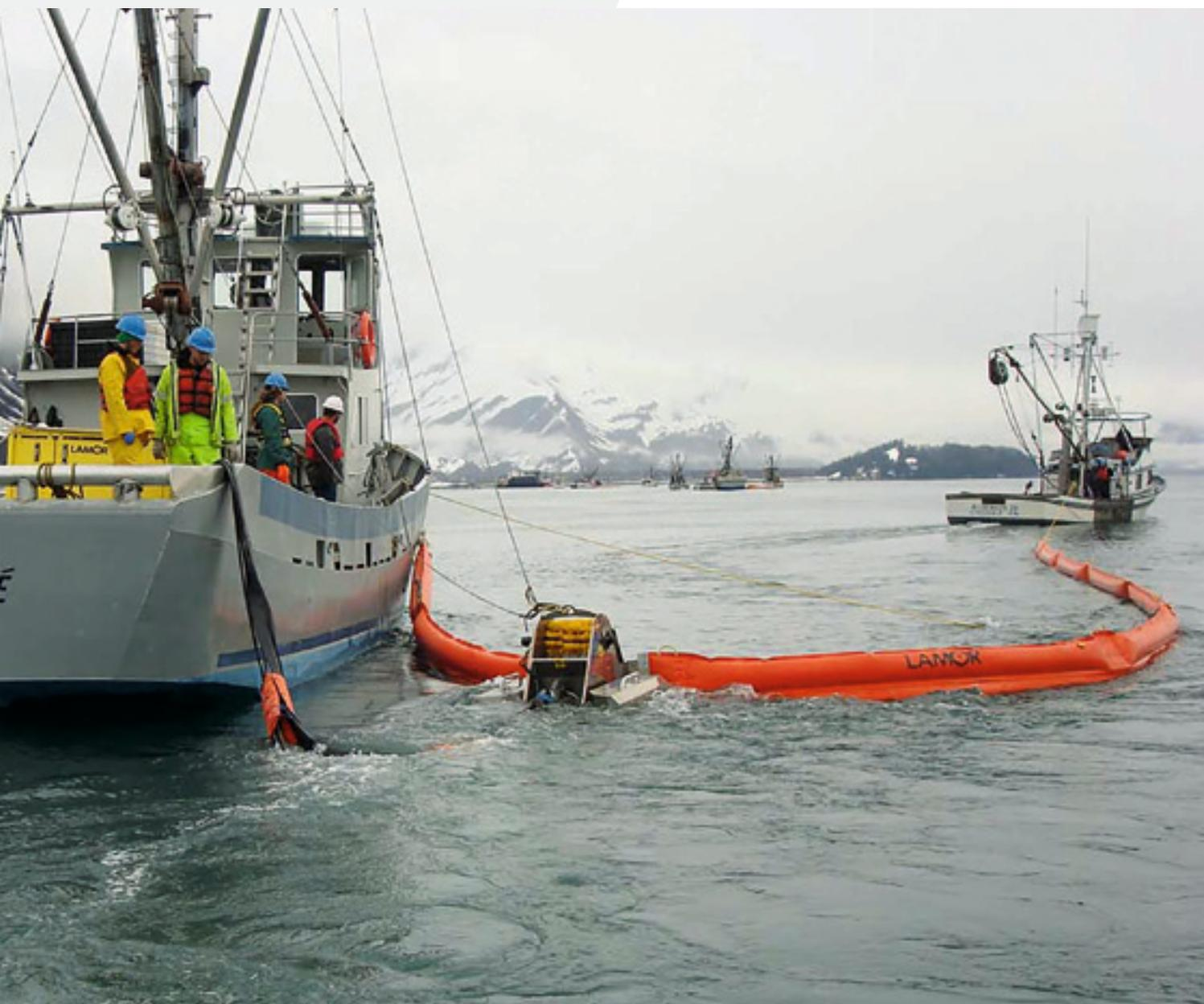
Multimax 50 (LAM 50), capacity: 50 m<sup>3</sup>/h (220 gpm)
