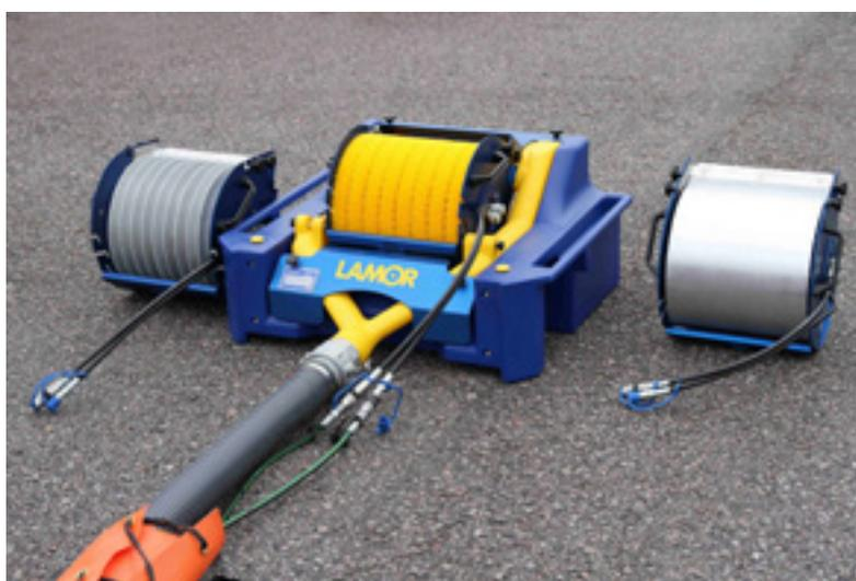
Minimax 25 (MM 25), capacity:  $25 \text{ m}^3/\text{h}$  (110 gpm)
