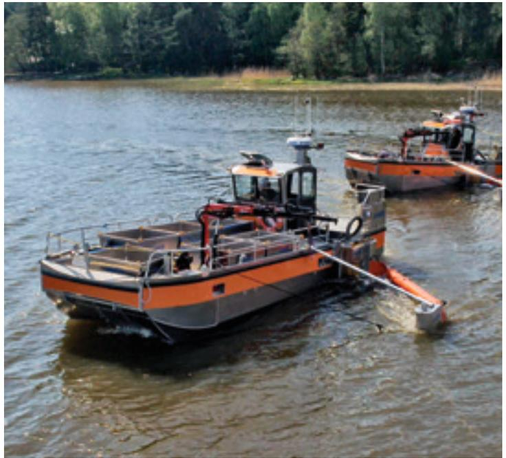
Ultra Shallow Draft Workboat equipped with side cassette for oil recovery
