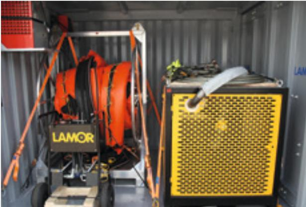
Containerized solution incl. power pack, hose reel and hydraulic control set for skimmers
