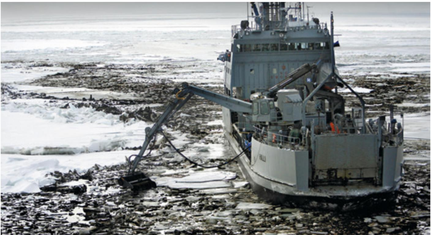
Bucket Skimmer (LRB 250), capacity: 140 m<sup>3</sup>/h (616 gpm)
