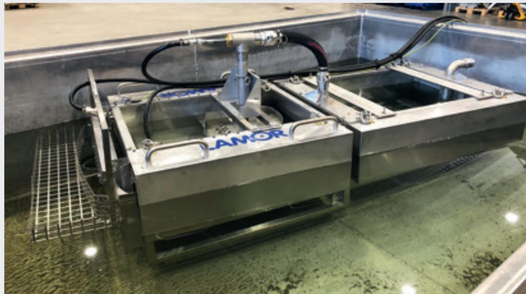
Industrial Process Skimmer Air (IPS A), capacity: 9.7 m<sup>3</sup>/h (43 gpm)
