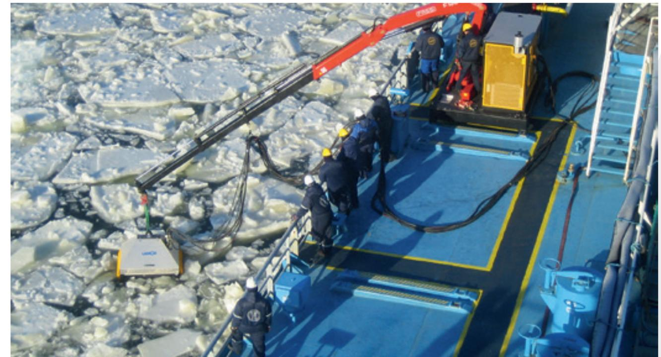
Arctic Skimmer 125 (LAS 125), capacity: 125 m<sup>3</sup>/h (550 gpm)
