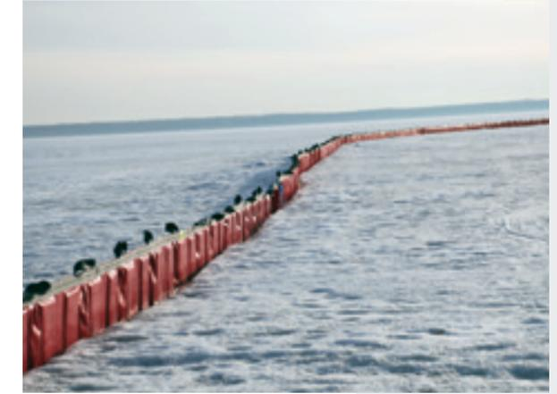
The FOB can also be deployed in ice conditions
