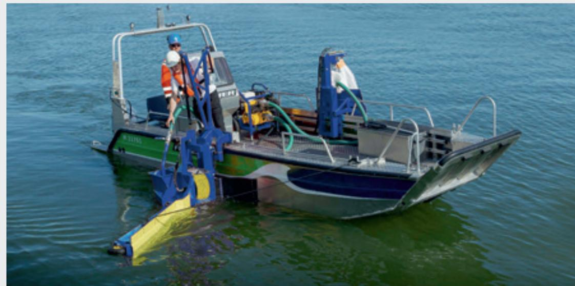
Side collector / MiniBagger, capacity: 10 m<sup>3</sup>/h (44 gpm)
