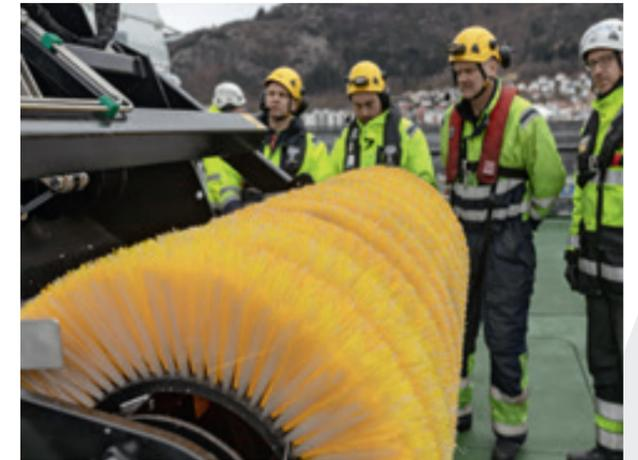
Vessel-mounted Bucket Skimmer (LRB 150), capacity: 115 m<sup>3</sup>/h (506 gpm)
