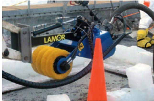
Lamor Recovery Bucket 40 (LRB 40), capacity: 19 m<sup>3</sup>/h (83 gpm)
