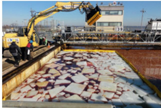
Bucket skimmer (LRB 150), capacity: 115 m<sup>3</sup>/h (506 gpm)
