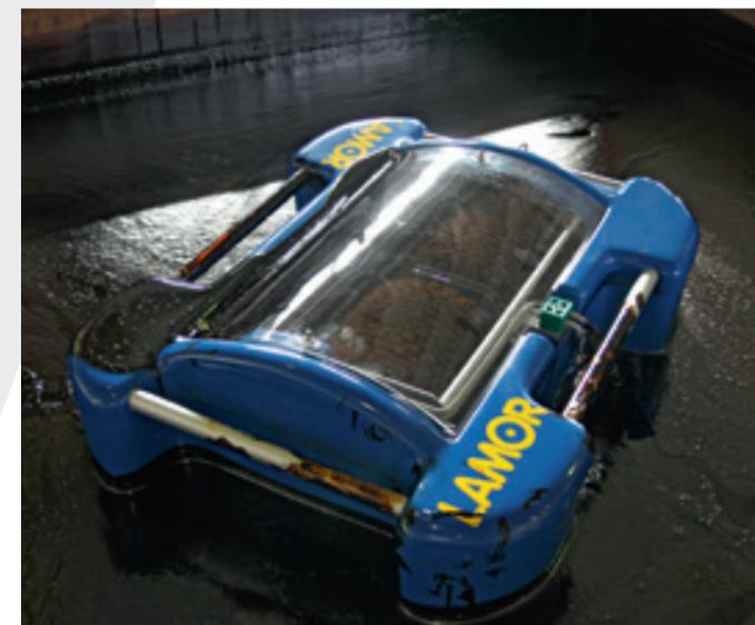
Minimax12 (MM12), capacity: 12 m<sup>3</sup>/h (52 gpm)
