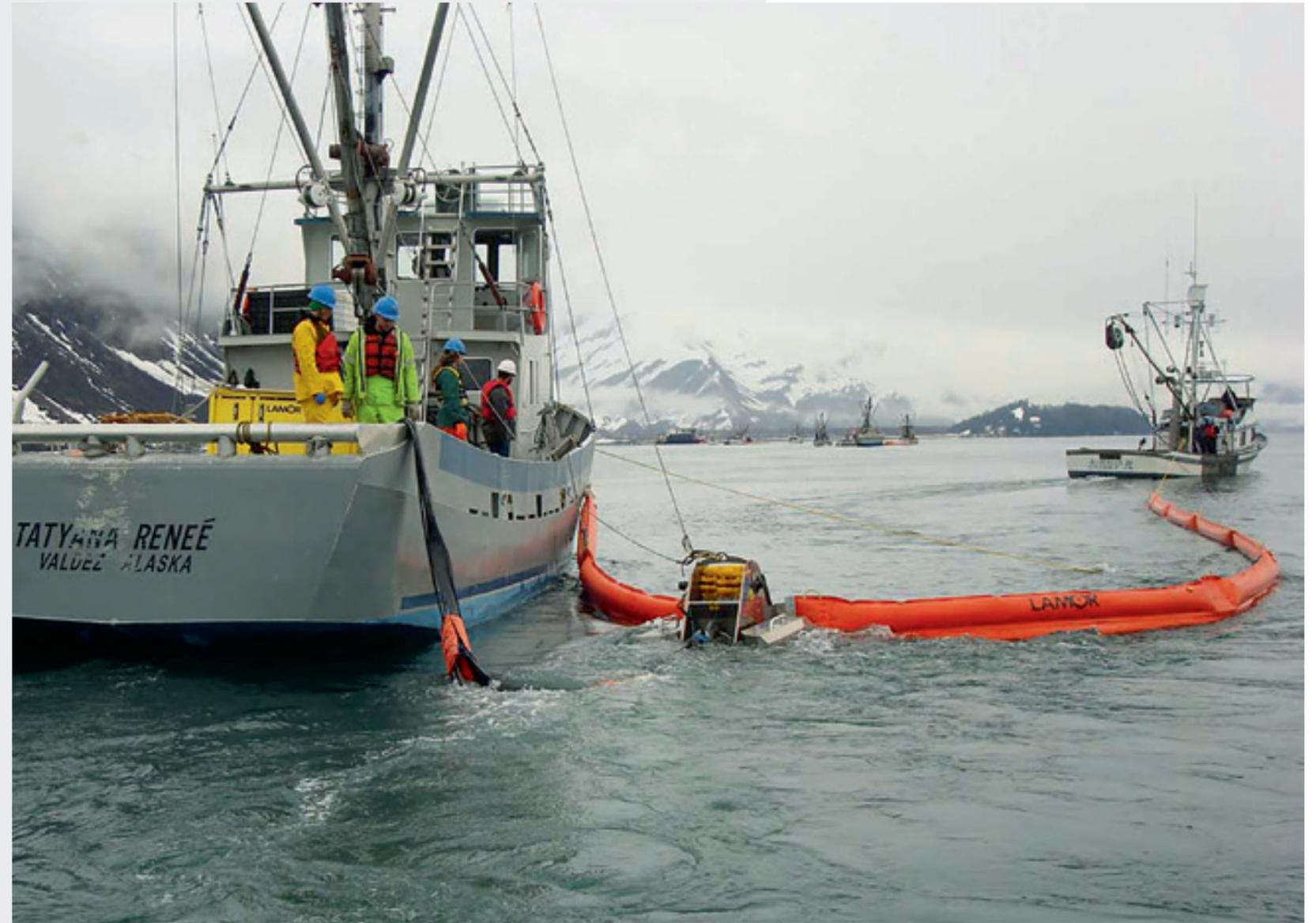
Multimax 50 (LAM 50), capacity: 50 m<sup>3</sup>/d (220 gpm)
