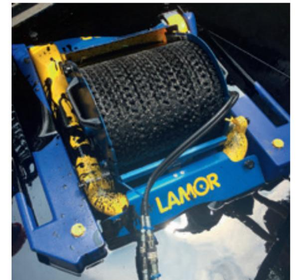
Mini max 25 (MM 25), capacity: 25 m<sup>3</sup>/h (110 gpm)
