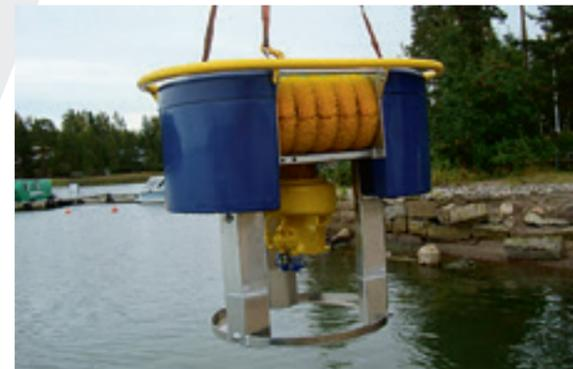
Multiskimmer (LMS 50/70), capacity: 271.5 m<sup>3</sup>/h (1,195 gpm)
