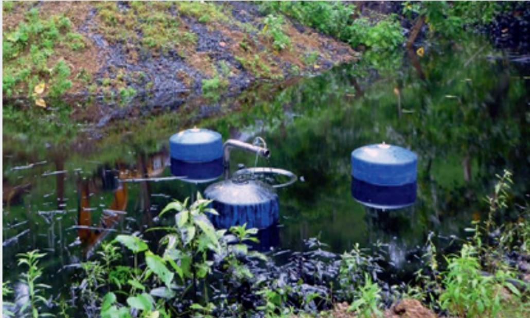
Weirskimmer 500, capacity: 70 m<sup>3</sup>/h (308 gpm)
