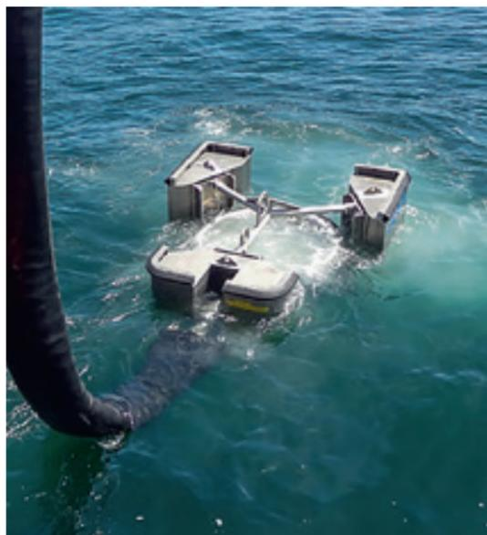
Weir Skimmer 1300 Brush (LWS 1300), capacity: 360 m<sup>3</sup>/h (1,585 gpm)
