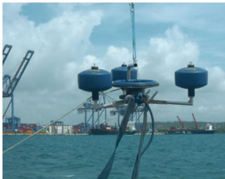
Weir Skimmer 800 (LWS 800) capacity: 112.2 m<sup>3</sup>/h (494 gpm)
