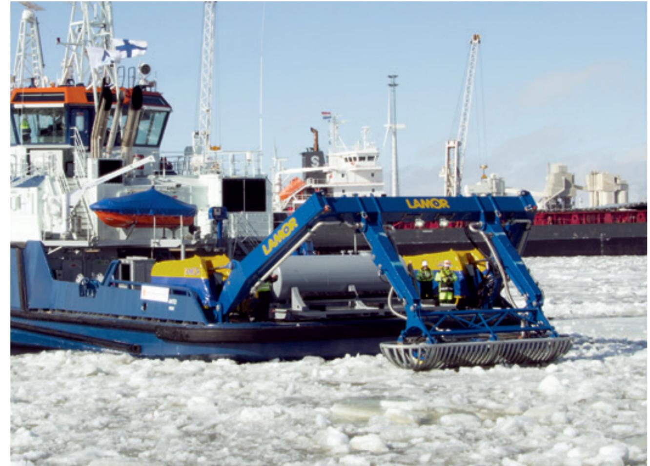
Sternmax, capacity: 560 m<sup>3</sup>/h (2,465 gpm)
