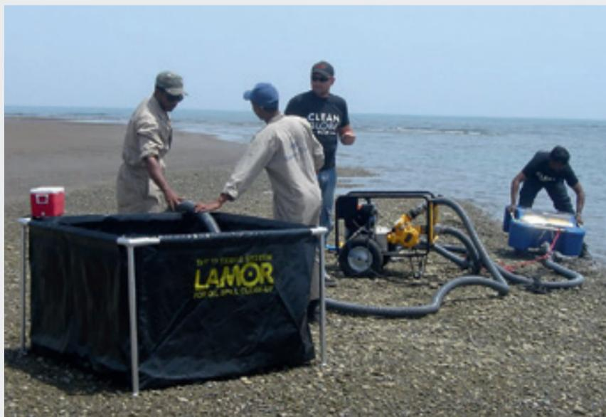
Collapsible oil storage tank, LPP 6 C 75 and Minimax 12 skimmer
