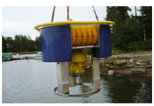
Multiskimmer (LMS 50/70), capacity: 271.5 m³/h (1,195 gpm)
