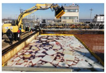
Bucket skimmer (LRB 150), capacity: 115 m<sup>3</sup>/h (506 gpm)
