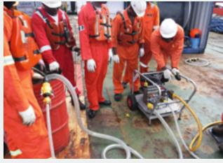
Deployment of dispersant system onboard vessel
