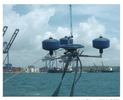
Weir Skimmer 800 (LWS 800) capacity: 112.2 m³/h (494 gpm)
